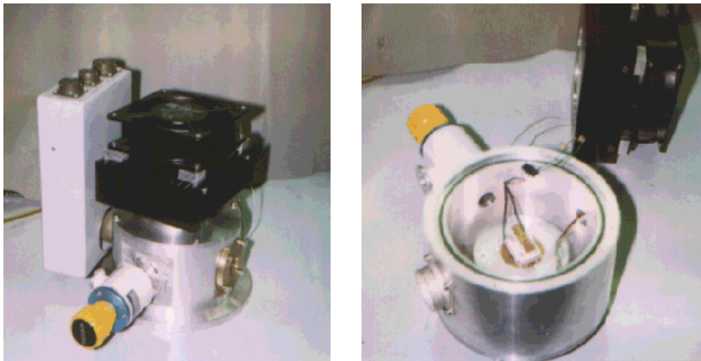
Figure 2 - Left panel: outside view of the preliminary version of the CCD housing, it is clearly visible the preamplifier box and the outside part of the cooling system. Right panel: inside view of the housing with the Peltier assembly.
