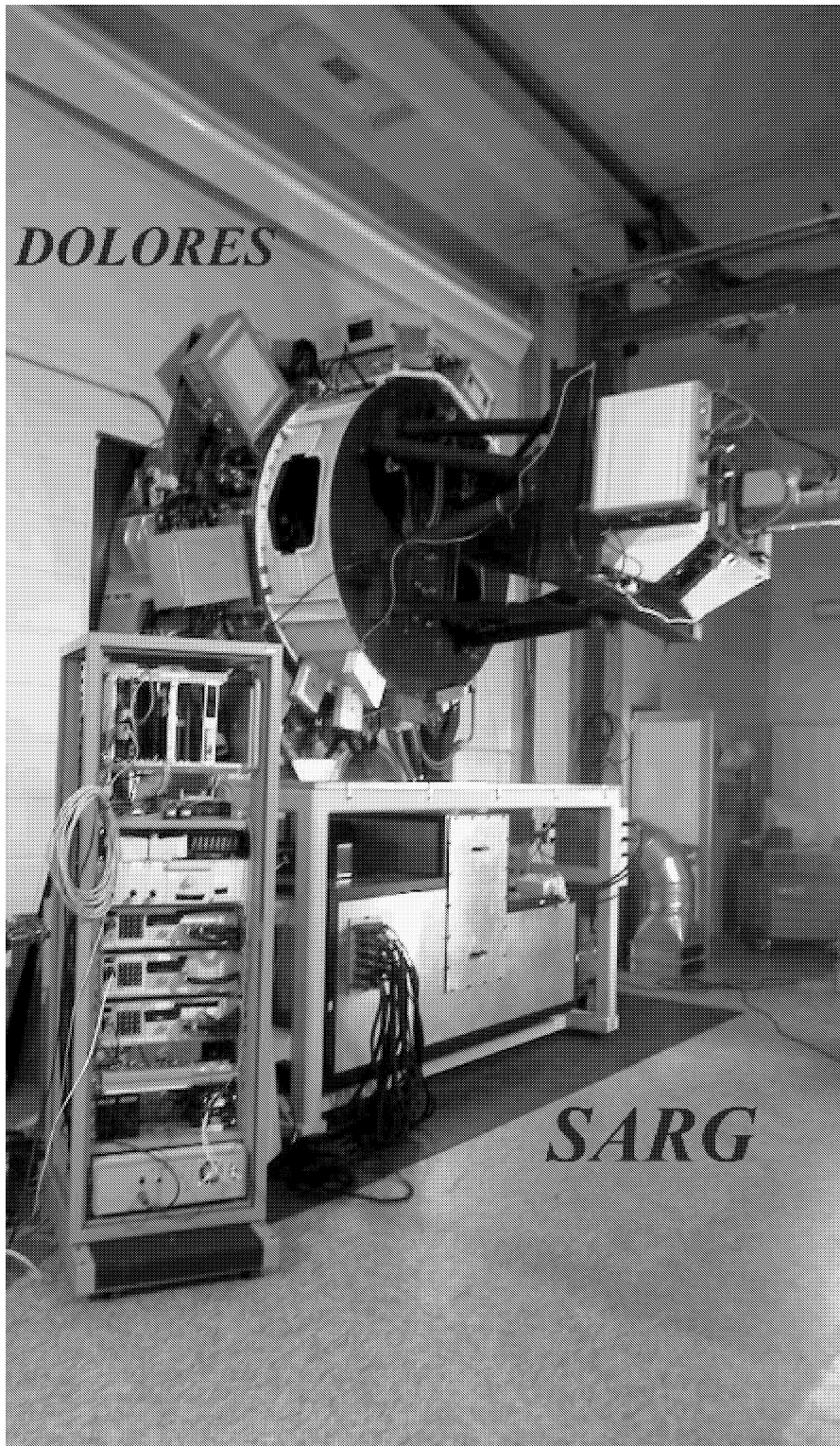
Figure 1. SARG layout in the TNG Nasmyth room B. On the foreground, the SARG electronic rack. Behind it, the SARG, rigidly mounted on the telescope fork. Light reaches the spectrograph from a folding mirror (in this picture hidden by the DoLoRes structure). The rotator adaptor is kept fixed when using SARG. Field derotation is achieved by means of an optical derotator. Guiding is done at the slit, using a cooled CCD.
