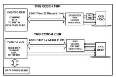
Figure 1. Block Diagram of the two CCD controller
