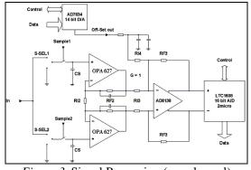
Figure 3. Signal Processing (one channel)
